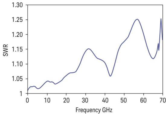
Typical SWR, 10 MHz to 70 GHz (25 ± 10 °C) for N8488A power sensor
